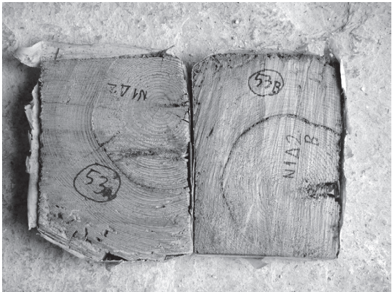
Fig. 3. Samples taken from both ends of beam no. 53, south wall, first floor (before sanding). The last preserved ring grew in AD 1327.
