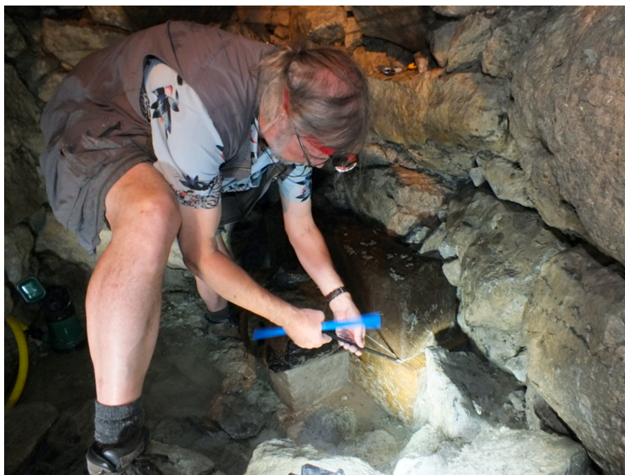
Fig. 6. Dendrochronologist Tomasz Ważny sampling the LBA wooden water-drain installation of the spring chamber of Oymağaç Höyük/Nerik with a 5 mm increment borer in 2019 (Photo: Oymağaç Project, D.P. Mielke).
